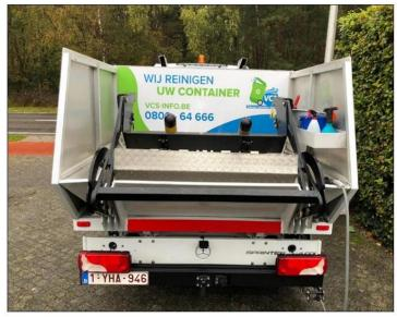
Rear view of the Mercedes Sprinter with the container lifting system in the transport position, both high pressure wash heads are visible in the middle, on the right side is positioned the chain with hose on the roller.
